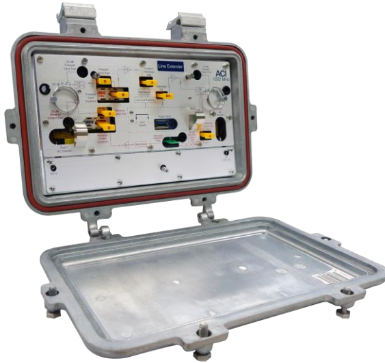
AFM-L (1 Output Line Extender)
