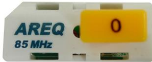
AREQ 85 MHz (JXP PLATFORM) For use in ASEM Moto, Cisco & C-Cor, and LEA1G (5-Pin) Reverse equalizers available from 0 to 12.0 dB in 1.0 dB steps by (Note. JXPXXX-XX.X sold separately)
