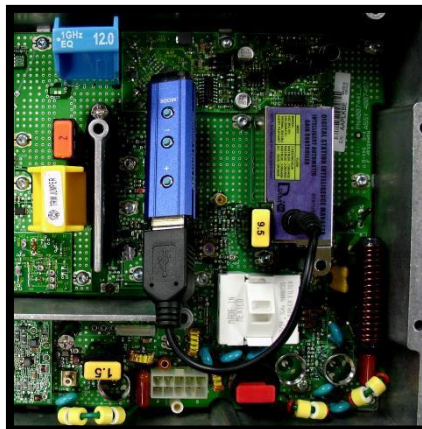
Controller Connection to DSIM (Shown with faceplate cover removed for clarity)
