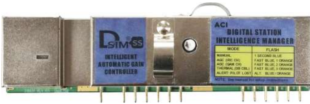
DSIM-SS for use in SA System Amplifiers P/N DSIM-SS-MDL-01 (without EQ) P/N DSIM-SS-MDL-02 (with EQ)
