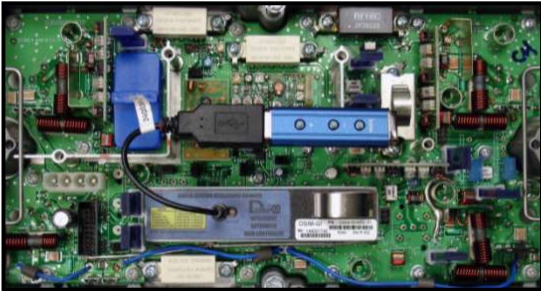
DSIM-GI AGC module with Interface cable attached to the DSIM controller
