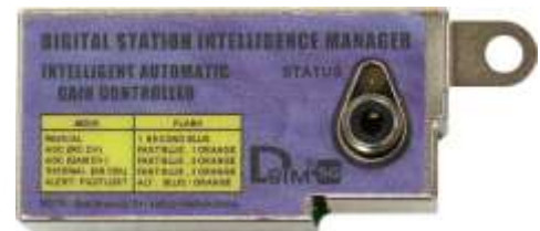
DSIM-SG for use in Scientific Atlanta® Amplifiers GainMaker P/N DSIM-SG-MDL-01
