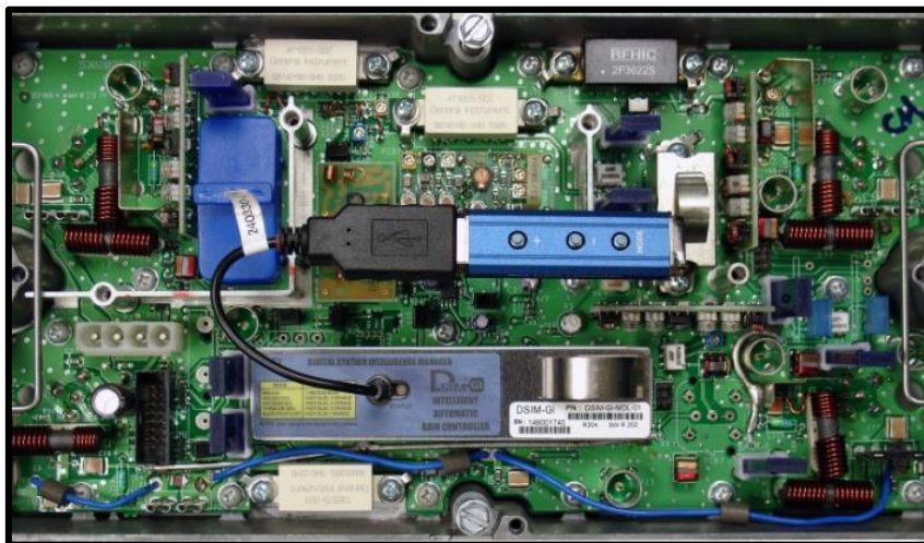
Controller Connection to DSIM (Shown with faceplate cover removed for clarity)
